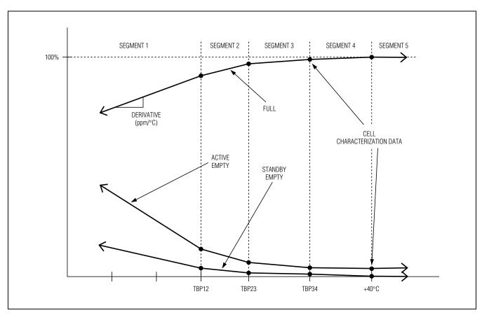
Figure 14. Cell Model Example Diagram
