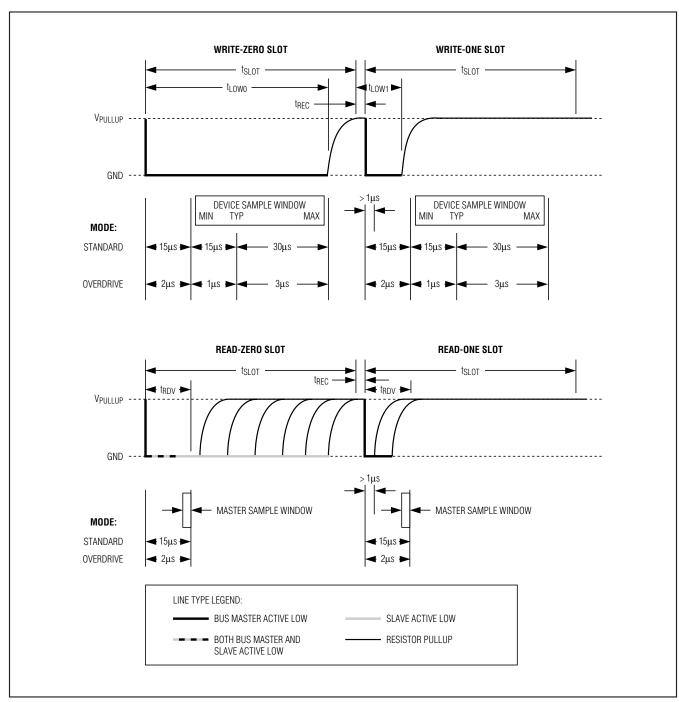
Figure 30. 1-Wire Write and Read Time Slots
