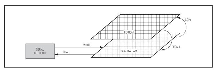
Figure 21. EEPROM Access Through Shadow RAM
