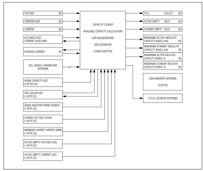
Figure 13. Top-Level Algorithm Diagram
