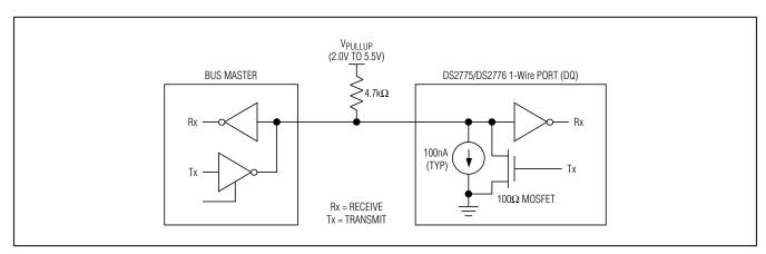
Figure 24. 1-Wire Bus Interface Circuitry
