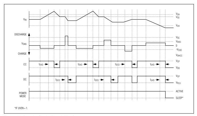
Figure 3. Li+ Protection Circuitry Example Waveforms
